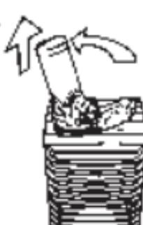
Put the edge of the Mouthpiece into the notch of the Rotary Cap and turn it counterclockwise to open and pull out. Pull off the Seal Ring from the Rotary Cap using the Filling Chamber Tool.
