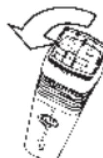
Unscrew the Cooling Unit Base from the Vaporizer by turning it 90° counterclockwise.
