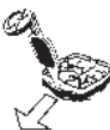
Lever out the large Base Seal Ring with Filling Chamber Tool at the recess in the groove.
