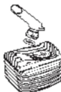
Pull the Mouthpiece out of the Cooling Unit Cap while slightly turning it counterclockwise. Pull off the Mouthpiece Seal Ring using the Filling Chamber Tool.
